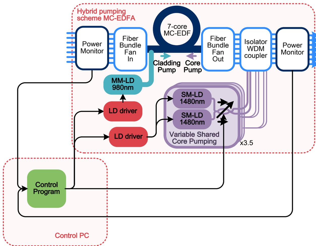
The most power efficient pumping scheme will depend on the signal allocation
