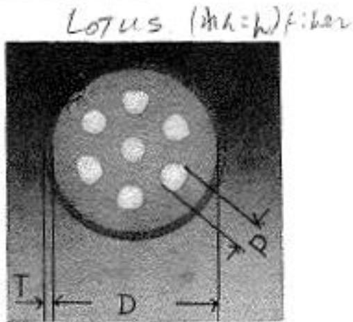
WB1 Fig. 3. Cross-sectional photograph of 7-core fiber:  $d = 23 \mu\text{m}$ ,  $D = 150 \mu\text{m}$ ,  $t = 5 \mu\text{m}$ ,  $\Delta = 1\%$ .
